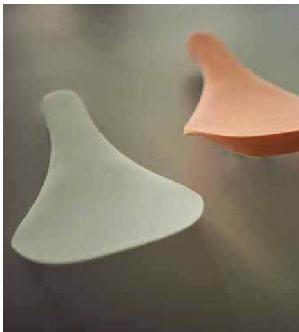
3D-Prints of the Seating shell and CNC-cut Foam Core
