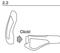
Fit the bar end to the grip. You will hear a distinct "click" when the integrated security ring engages. This signals that the bar end is properly fitted to the grip.
