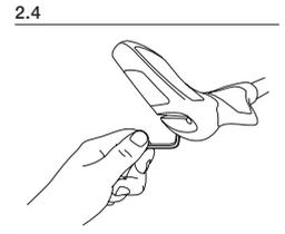
Tighten the clamping screw so that the grip and bar end can still be moved.
