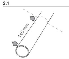
Measure and mark the handlebar 140 mm from the end. Tipp: Use either sticky tape or a pencil.
