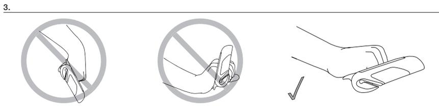
Turn the grip so that the support platform completely supports the ball of your hand. The wrist should be in a neutral position avoiding an exaggerated kink. After a short period of trial and error a comfortable position can be found. Be sure to tighten the clamp with 7 Nm before your first ride.
