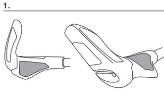
The grips are left and right specific, please ensure that they correctly orientated.
