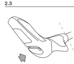
Push the grip and bar end on to the bar as far as the 140 mm mark.
