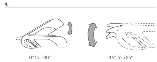
The default position for the support platform is horizontal. For fine tuning according to rider and riding style, please refer to the step 3 and the tips given below.
