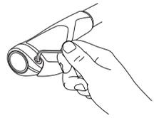
Tighten the clamp using the upward facing screws.
