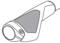
Slide the grip onto the handlebar.
