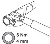
Tighten to 5 Nm torque using a 4 mm torque wrench. Re-check the torque setting following the first ride / 50 km of riding. Check periodically to ensure that the screws are not loosening.
