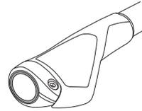
Ensure that the grip is fully inserted onto the bar so that it is flush with the end of the bar.
